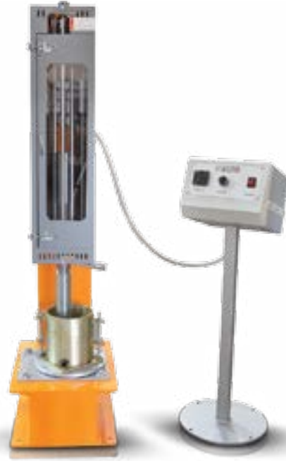
Automatic Soil Compactor (T-055)
