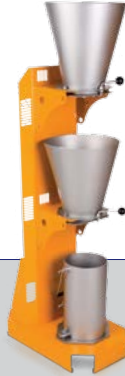
Compacting factor apparatus (B-185)
