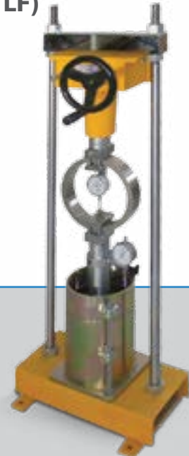
Field CBR (T-005) with Conversion Frame (T-005/LF)
